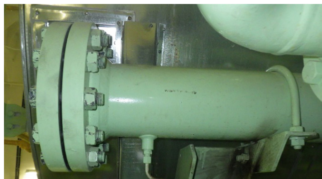
Fig. 3: Drain/venting pipe at starting air manifold at blind end (lowest point of starting air manifold).
