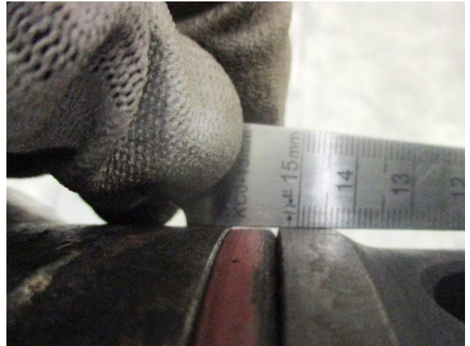
Fig. 6: Example of an O-ring with no sealing effect in the starting air valve. Please note the light between O-ring and steel ruler, which indicates that there is no sealing effect.
